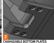
Operator can change wear plate easily
